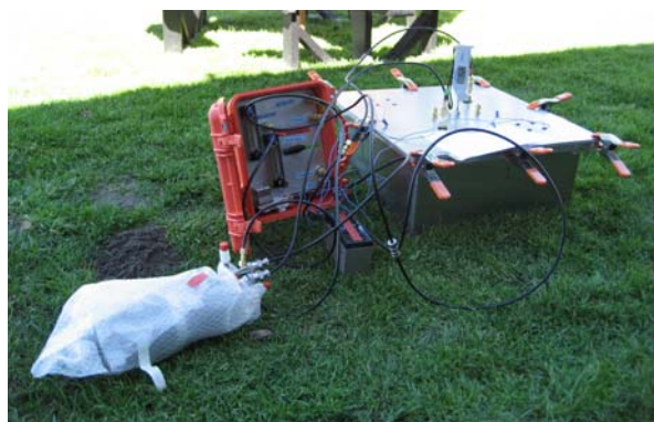
Figure 2. Surface N 2 flux chamber, pumping module, and flask (in bubble wrap).
